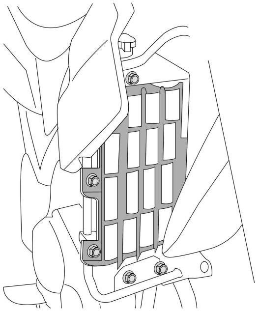
The Original Radiator Guard in motorbike is shown in the drawing.
