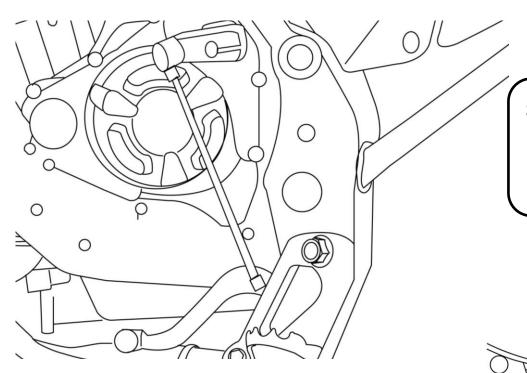
SRC Frame Protector uses the mounting hole located (as shown in the drawing). The Protector shields the frames (Left side)
