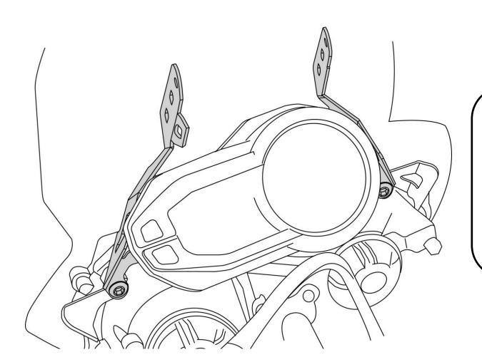
The LH and RH GPS Brackets in "As is mounted condition" is as shown in the drawing to the right.
