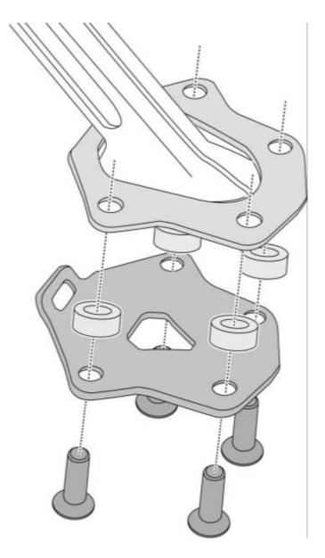
Slip-in Countersunk Screw M6 x 20 (5) – 4 off from the bottom side of the Bush Spacer (4) the Lower Plate (1), as shown.
