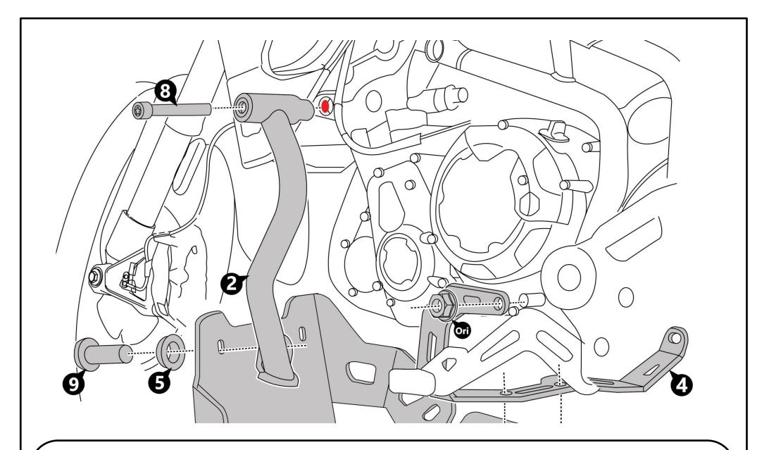
Orient and Align the Bracket bar LH (2) Slip – in screw M10 X75 (8), in-line to the 1 off mounting holes (red color as show in the motorbike). And Orient and Align the Bracket Lower (4) Slip-in the original Nut-1 off , and secure the threads in the bracket, as shown.
