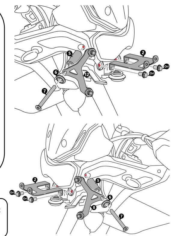
Repeat the Step 4 for mounting the Bracket LH (5), as shown
