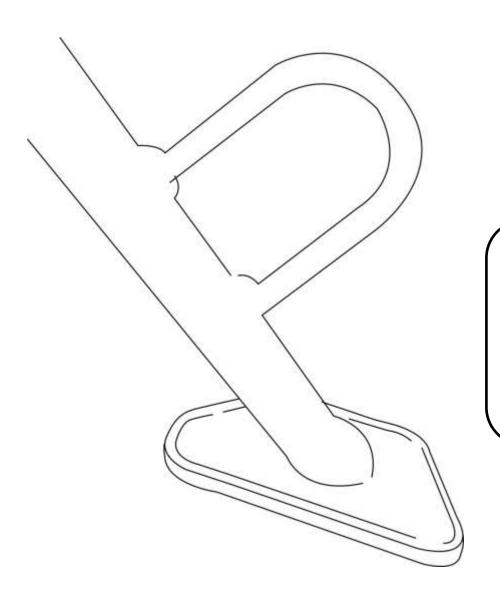
The Motorbike has to be held using the central stand, and Side Stand, drawn to the sides, to have access to the mounting of Large Side stand.
