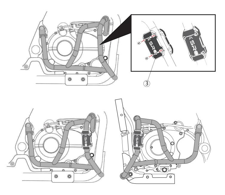
Please tighten the bolts to the recommended value/NM/ and insert/lock thread/ according to the instructions.
