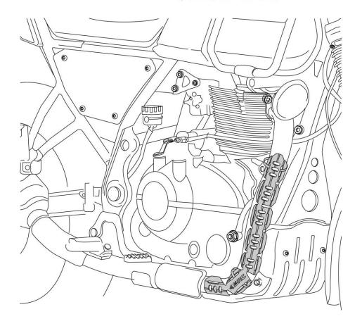
Align and Orient the Metal Cover along the Exhaust Pipe and securely tag it using the Circular "C" Metal clips clinging to the Exhaust Pipe, one at the top and the other at the bottom, as shown in the drawing
