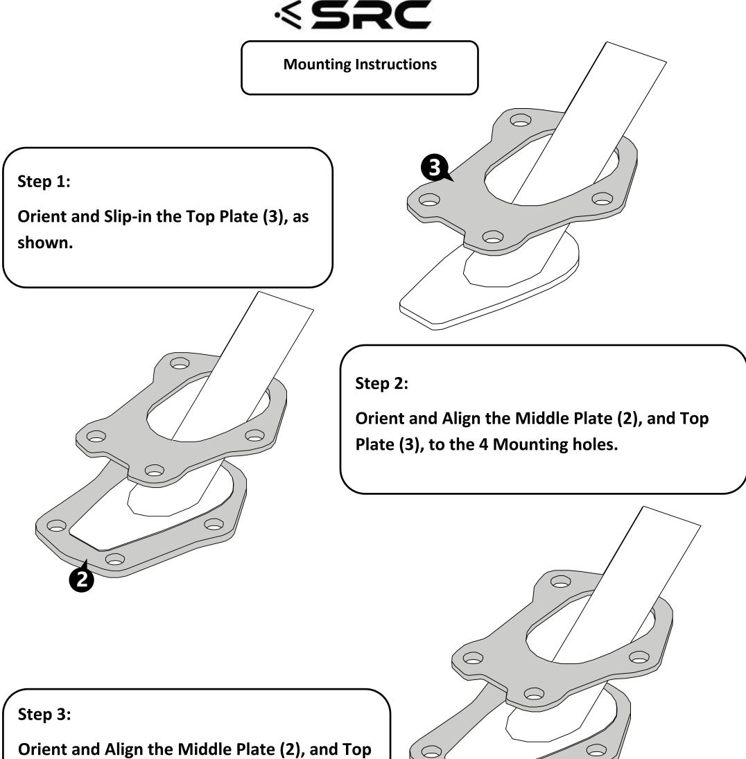
Plate (3), and Low Plate (1) to the 4 Mounting holes.
