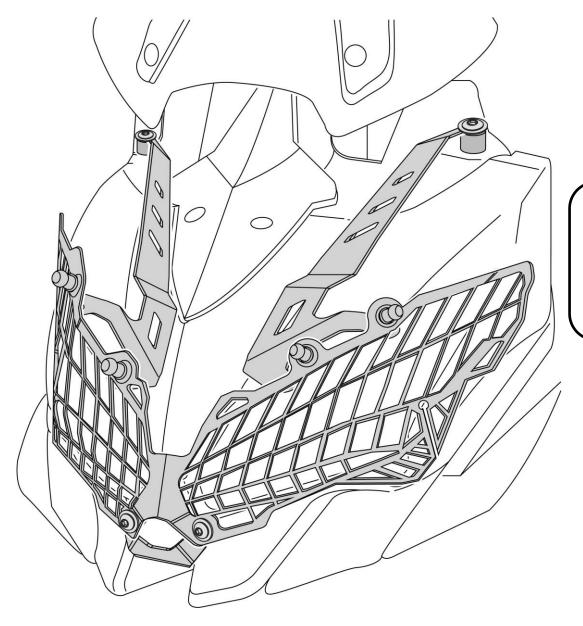
The Installation of the Head Light Guard is complete and is as shown
