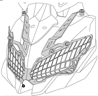
"As is mounted condition" of Head Light Guard is as shown in the drawing to the right.
