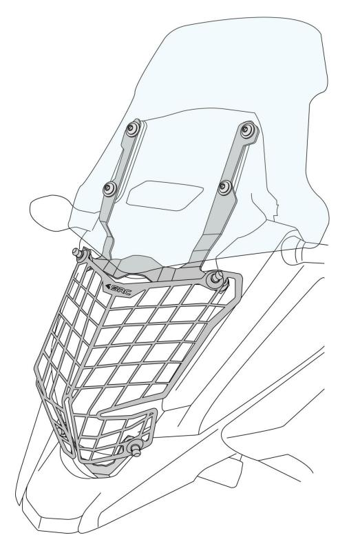
Final Mounted condition of the Head Light Guard is as shown in the above drawing.
