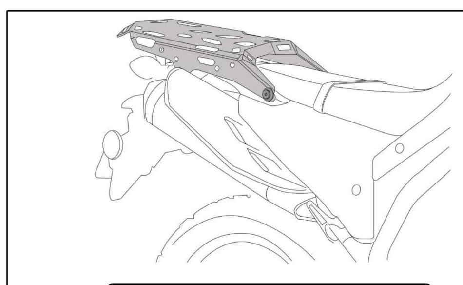
The Top Rack in "As is mounted condition" is as shown.
