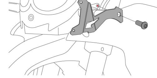
Orient and Align the Bracket LH (3) and secure the threads in the Mounting Hole (shown in red colour) behind the Indicator Lamp, using the OE screw, which was removed in the previous step.
