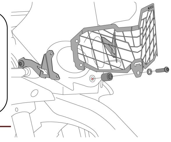
shown, and secure the threads in the Mounting hole (shown in Red colour), beneath the Head Light, and tighten them fully to the torque, as specified in the BOM table.
