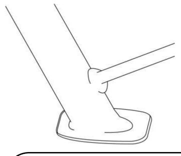
The Motorbike has to be held using the central stand, and Side Stand, drawn to the sides, to have access to the mounting of Large Side stand.
