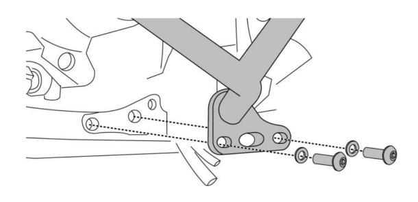
Lateral Side Bracket – RH in "As Is Mounted Condition"
