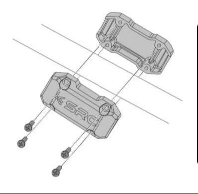
Assemble the Slider Bar on each of the Crash Bar as shown.
