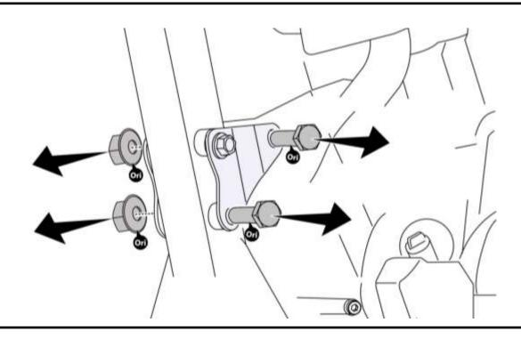
Remove the Original screws and Nuts from the original frame at front.
