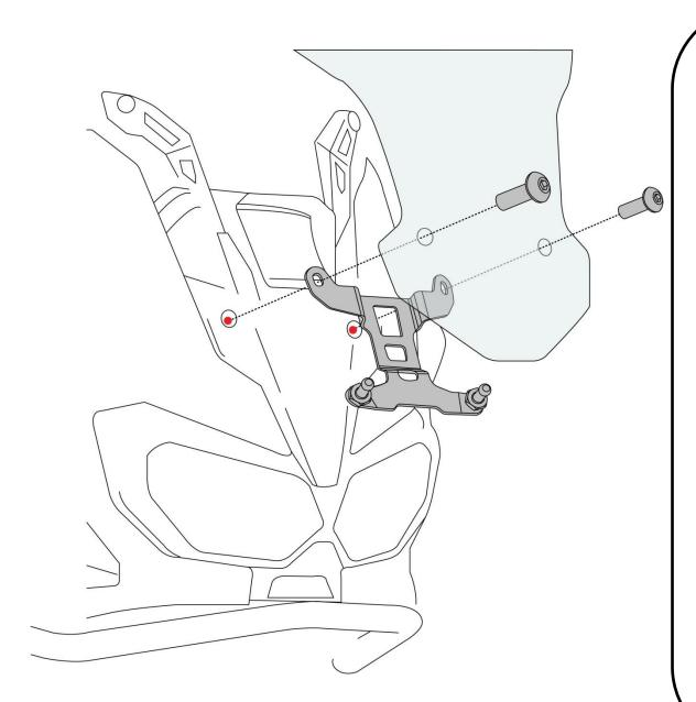
Step 3: Mounting the Upper Bracket (2) and the Windshield Guard (back in its position)
