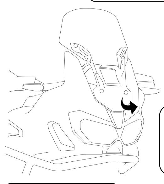
Step 1: Unscrew the two mounting screws of the Windshield Guard to enable access and fitment of the lower bracket (3)
