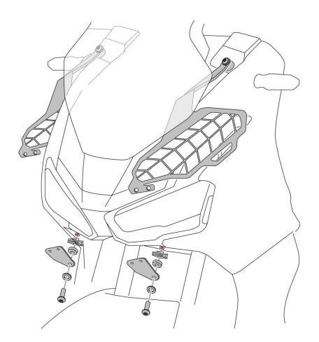
Mounting of the Bottom Plate LH (2).& the Bottom Plate RH (6) This takes the mounting hole available in the Motorbike (as shown in the drawing).
