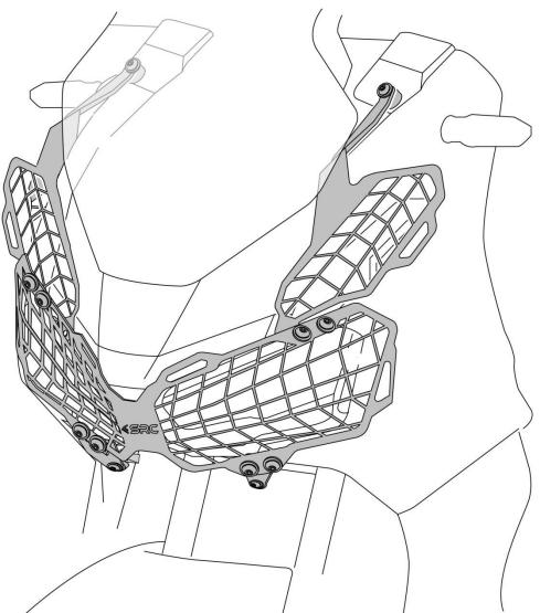
Ensure Mounting symmetry and tighten the screws to torque as per specifications in the BOM table.
