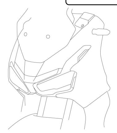
The Mounting Screws, which will be used for mounting the Brackets of the Head Light Guard, can be found on the Front Left hand side and Right hand side. The same can be unscrewed out, 2 off on each side.
