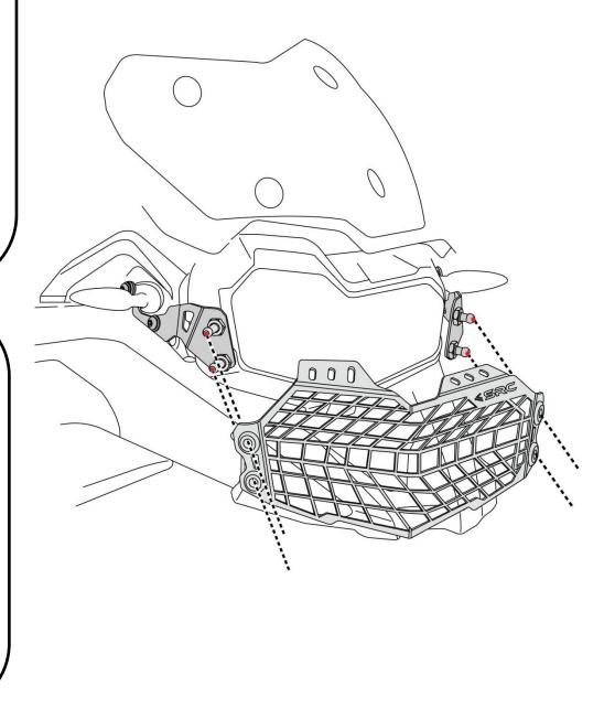
Orient the Head Light Guard (1), as shown. Assemble the Grommet (4) – 4 off, hugging and flush, with the outer surfaces of the Head Light Guard.
