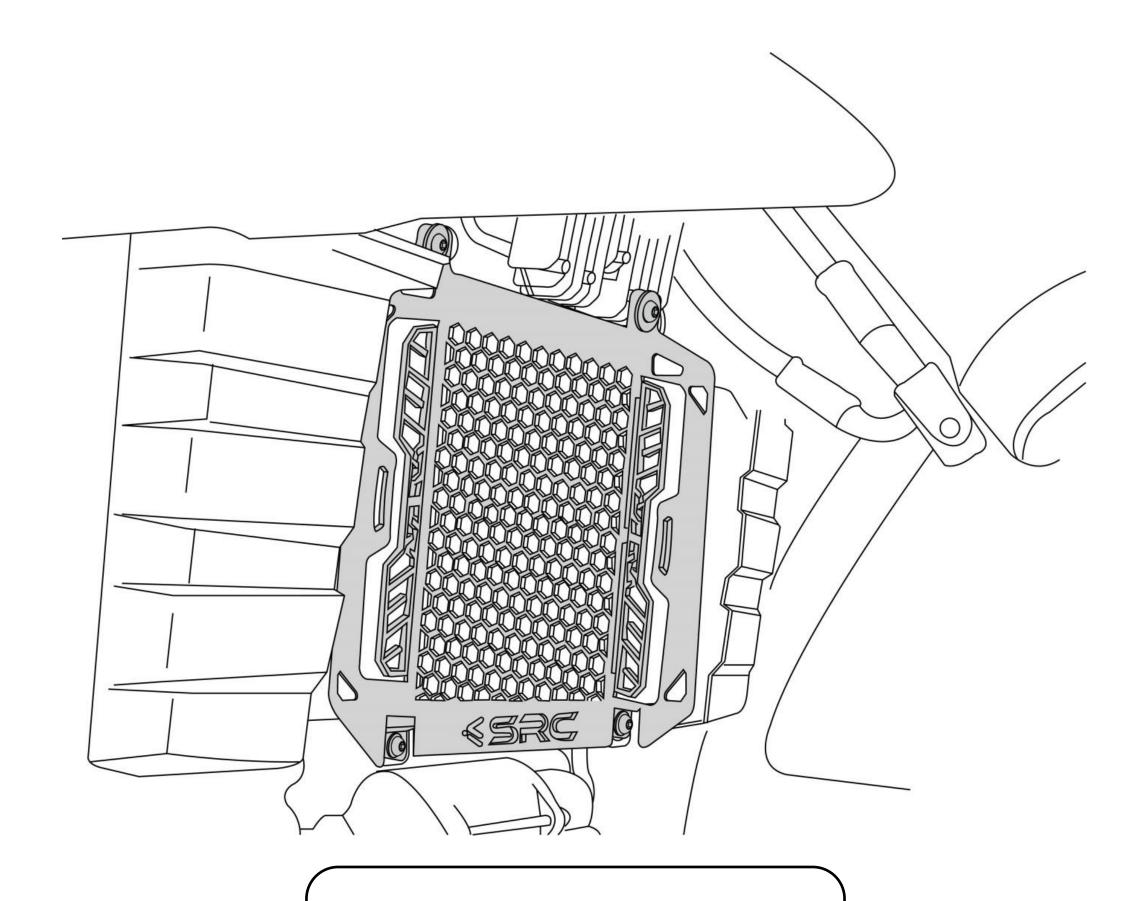
Final mounted condition of Radiator Guard, is as shown in the drawing.
