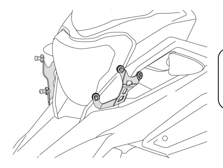
Bracket RH & Bracket LH is shown in "As is mounted condition"
