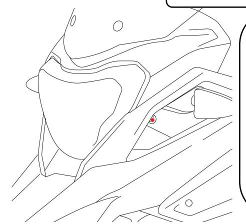
The Mounting hole, which will be used for mounting the Brackets of the Head Light Guard, can be found on the Front Left hand side and Right hand side.
