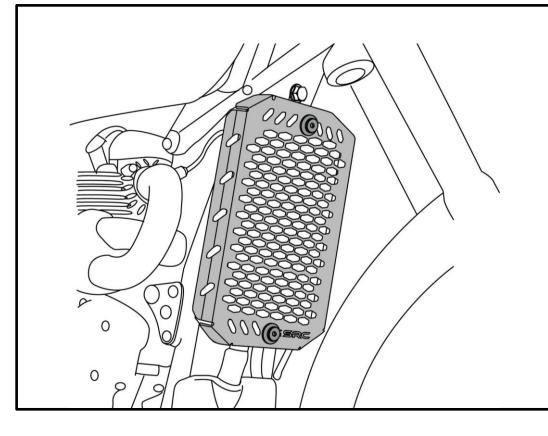
Radiator Guard in "Final Mounted Condition"
