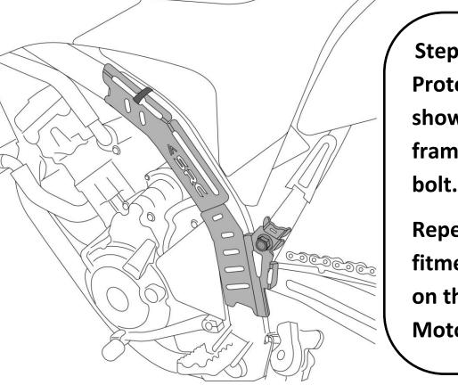
**Step 3: Ensure visually the Protector shields the Frame, as** shown and tie-up the cable to the frame at the top and tighten the
