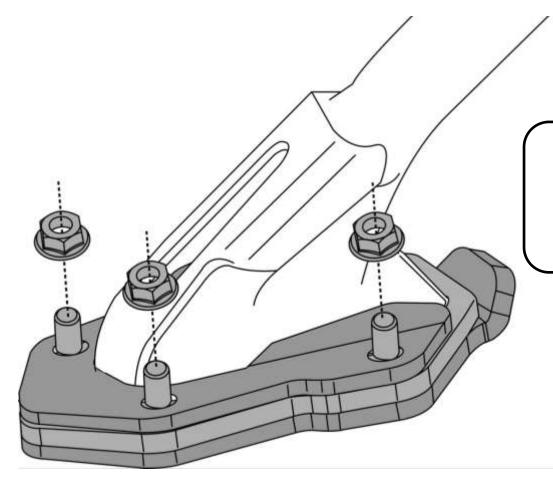
Secure the threads on the screw using M6 Nut (5), as shown.
