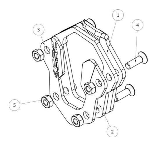
\*\*Deno tes Usage of Liquid Thread Locker in specified Locations
