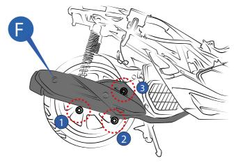
8 Remove the standard shock absorbers by loosening the upper nuts and lower mounting bolts ①②
