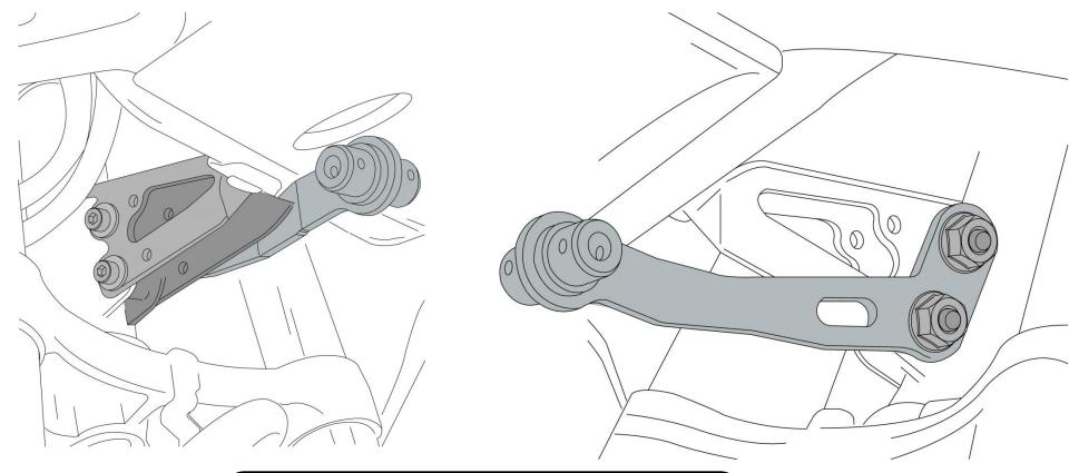
As is Mounted condition of the mounting the Upper Plate is as shown.
