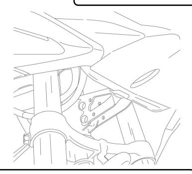
The Mounting Holes for mounting the Upper Plate (5), can be found in-between the front forks and positioned inside, and it is part of the Motorbike Chassis frame.
